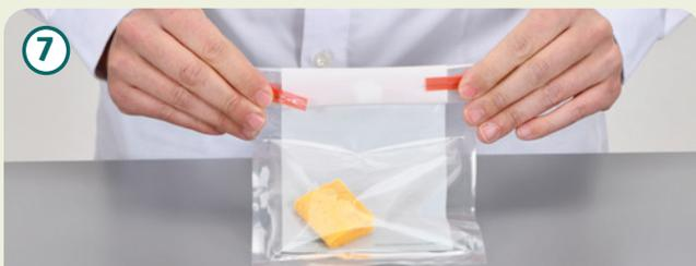
Use the attached tie to close the Twirl-Tie™ bag by rolling the opening of the bag and then kinking the tie to the inner side.
