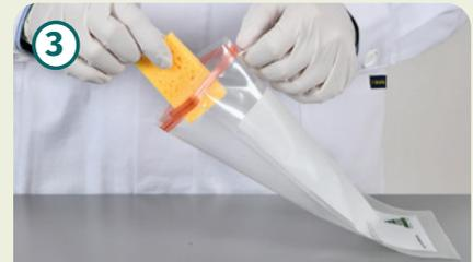
3 Put sponge into the sterile sample bag (or back into the vial) and label bag with sample details. Always switch gloves between sampling sites.
