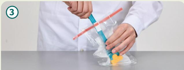
Pull the bag down from the outside to release the stick. Do not touch the stick lower than the thumb stop in the middle or the inner surface of the bag.
