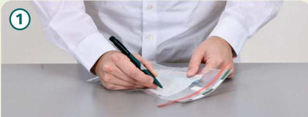
Label the bag in the white area. Ballpoint pens can be used. This sampling procedure does not require gloves!
